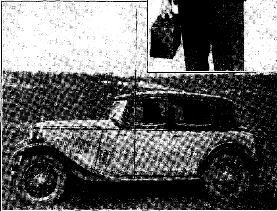
A 7ft. vertical copper rod serves as transmitting and receiving aerial for a car installation. A multiple cable connects the "transceiver" unit to the battery box.
