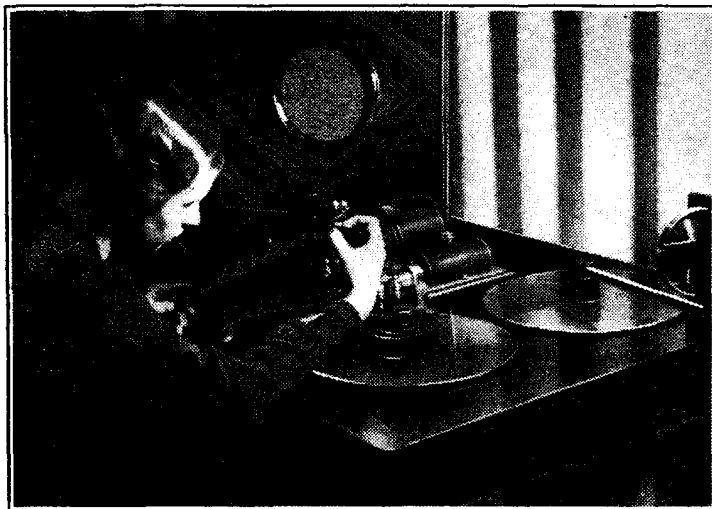
PROGRAMMES FOR TELEVISION. Regular transmissions of high-definition television are now made from the Berlin Broadcasting House, the programmes being changed once a week. The photograph shows the film-cutting table.
